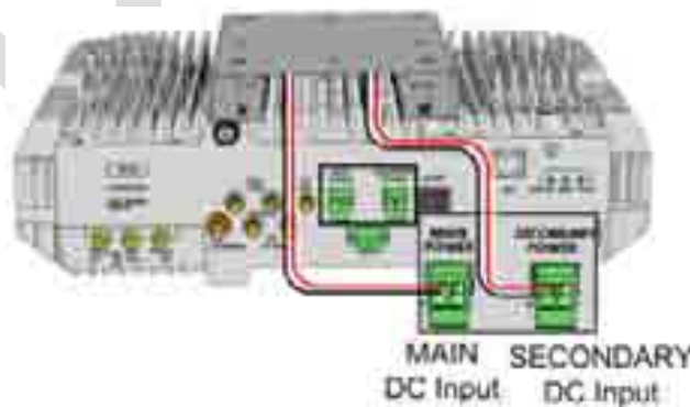
Figure 5-94. RAU5 MAIN and SECONDARY DC Input Connections
