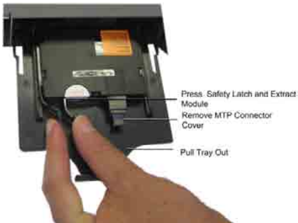
Figure 5-61. Extracting Edge Module
