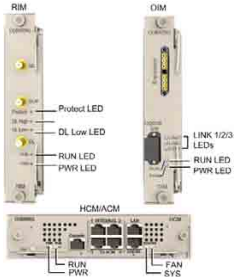
Figure 5-55. RIM, OIM and HCM/ACM LEDs
