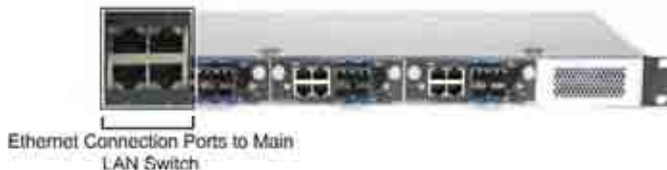
Figure 6-2. CEM LAN and Fiber Connection Ports
