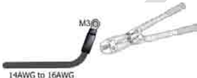
Figure 5-17. Crimping the Terminal Rings onto the DC Wire
