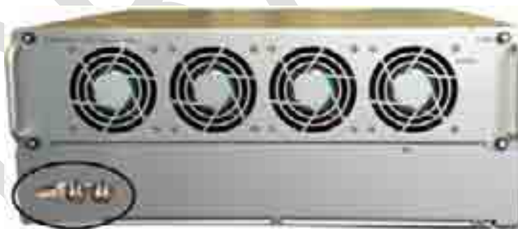
Figure 5-27. OIU Grounding Lug (Chassis Rear)
