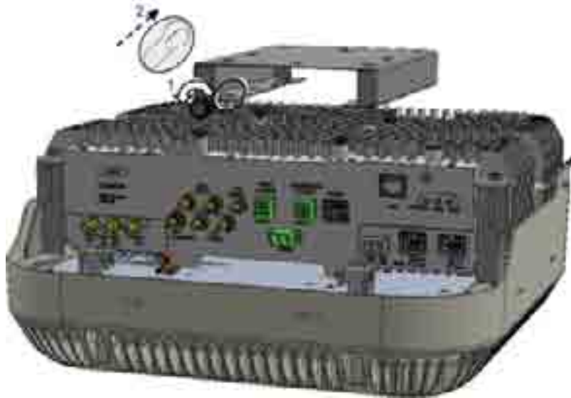
Figure 10-2 Removing Bracket and Antenna Skirt
