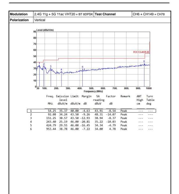
Note 1: Emission Level (dBuV/m) = SA Reading (dBuV/m) + Factor\* (dB)
