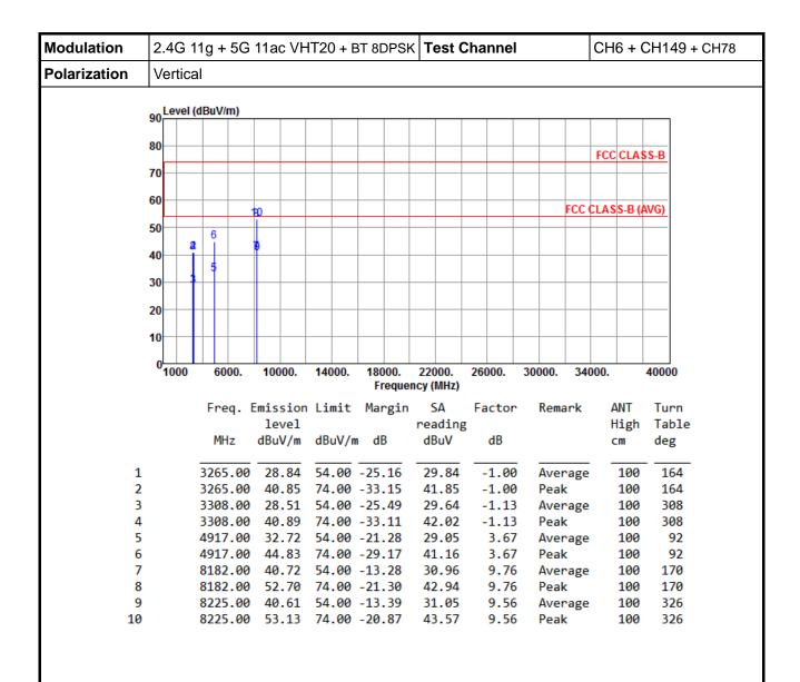
Note 1: Emission Level (dBuV/m) = SA Reading (dBuV/m) + Factor\* (dB)
