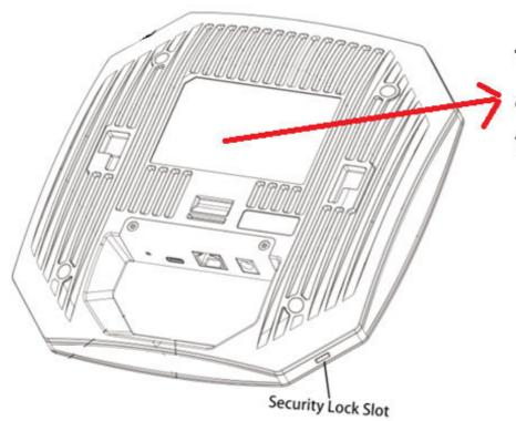
The label with FCC ID will be attached here on the bottom of the AP.
