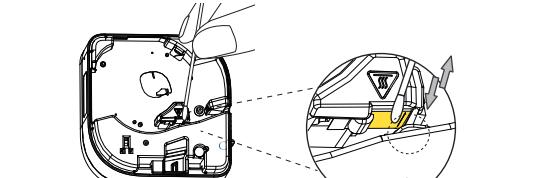
① Please avoid scraping the Print Head with any hard objects, as it may cause damage to the Print Head and worsen print quality.
