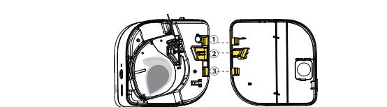
08 Push the Top Cover inward until it clicks, which indicates that it has been securely closed. Ribbon installation is now completed.
