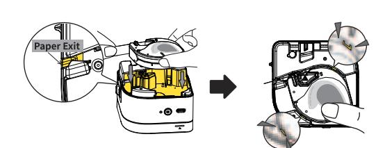
07 Align the Top Cover clasps with marked holes ①②③ on the Main Body.
