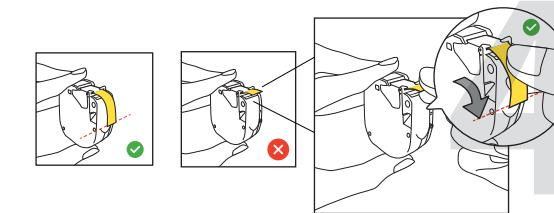
06 Place the label ribbon into the Ribbon Compartment and feed the extended ribbon into the Paper Outlet; then press down on the label ribbon until you hear a click, indicating the installation is complete.
