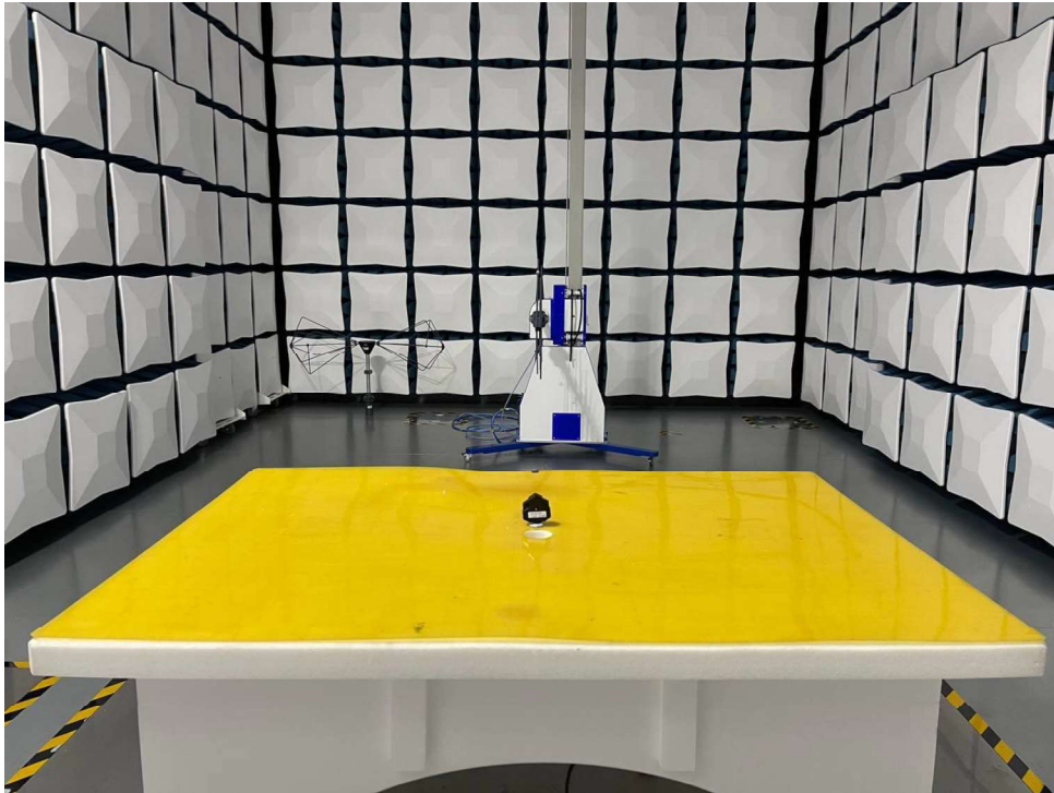
Set-up for Radiated Emission (200-1000MHz)
