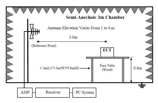
8.2.2. In 3m Anechoic Chamber Test Setup Diagram for frequency above 1GHz
