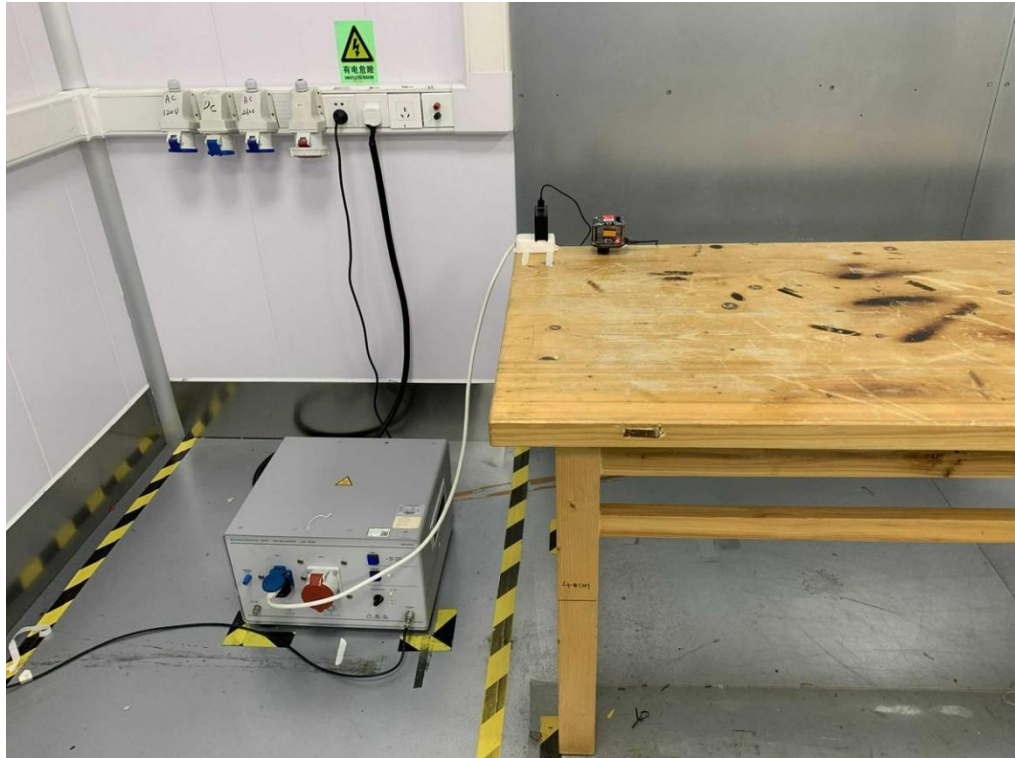
Conducted Emission at AC power line
