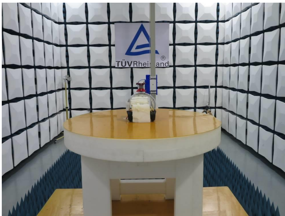
Photograph 2: Set-up photo for Radiated Spurious Emission, Above 1GHz
