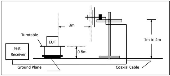
(c) For radiated emissions above 1000MHz
