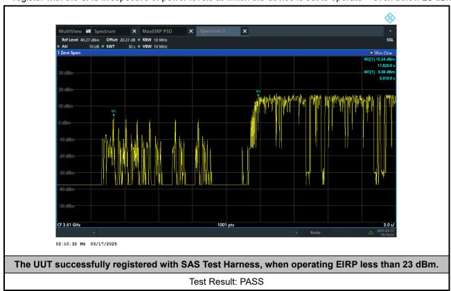
Note: The total offset 20.27 dB includes the antenna gain 7.2 dBi and cable path loss 13.07 dB.
