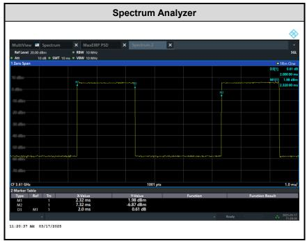
Note: The duty cycle value is 40%, add 10log(1/duty cycle) to the measured power level to compute the average power during continuous transmission.
