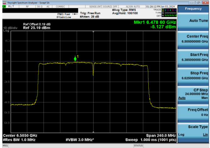
Plot 7-280. Power Spectral Density Plot Antenna WF2a LPI (160MHz 802.11ax (UNII Band 6) – Ch. 111, MCS2)
