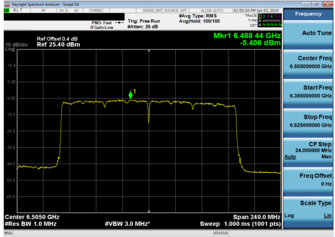
Plot 7-316. Power Spectral Density Plot Antenna WF2a LPI (160MHz 802.11ax (UNII Band 6) – Ch. 111, MCS11)
