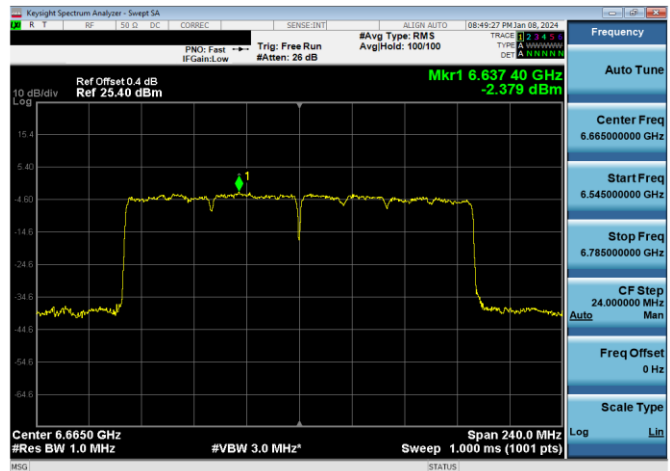
Plot 7-270. Power Spectral Density Plot Antenna WF7a Standard Power (160MHz 802.11ax (UNII Band 7) – Ch. 143, MCS11)
