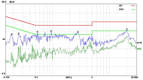
Site Chamber #2 Limit: FCC Part 15B Class B Conduction(QP)
