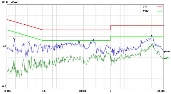
Site Chamber #2 Limit: FCC Part 15B Class B Conduction(QP) Phase: AC 120V/60Hz
