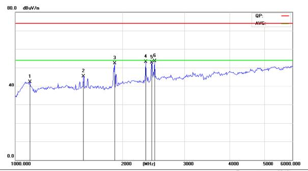
Site Chamber #2 Limit: FCC Part 15B Class B Above 1GHz RE(PK) Polarization: Vertical AC 120V/60Hz
