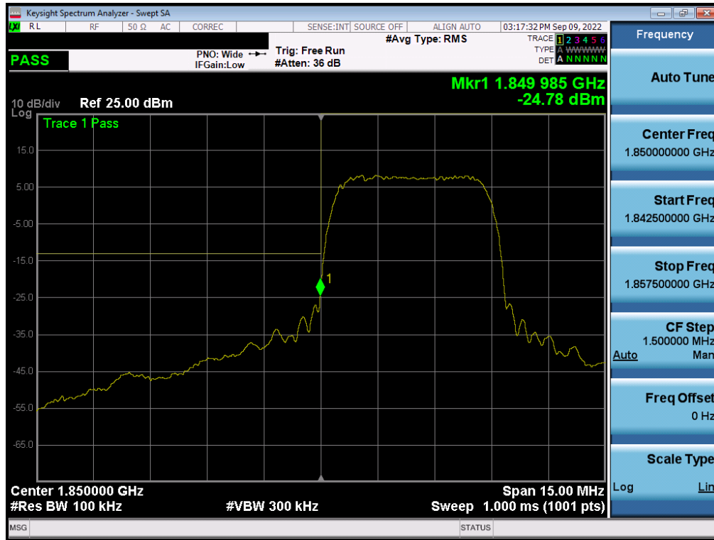
Plot 7-270. Lower Band Edge Plot (WCDMA PCS – Ch. 9262 - ANT A)
