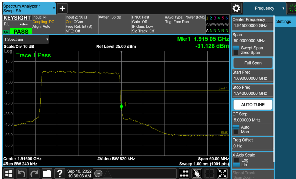
Plot 7-212. Upper Band Edge Plot (NR Band n25 - 20MHz QPSK – Full RB - ANT A)
