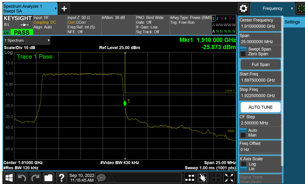
Plot 7-222. Upper Band Edge Plot (NR Band n2 - 10MHz QPSK – Full RB - ANT A)
