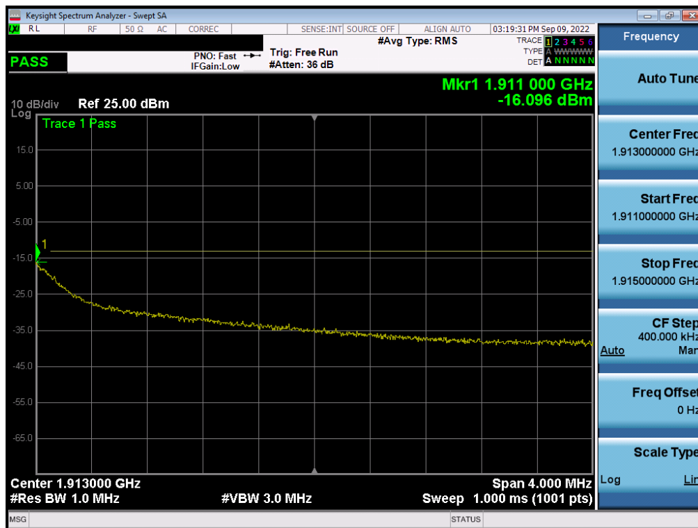
Plot 7-273. Extended Upper Band Edge Plot (WCDMA PCS – Ch. 9538 - ANT A)
