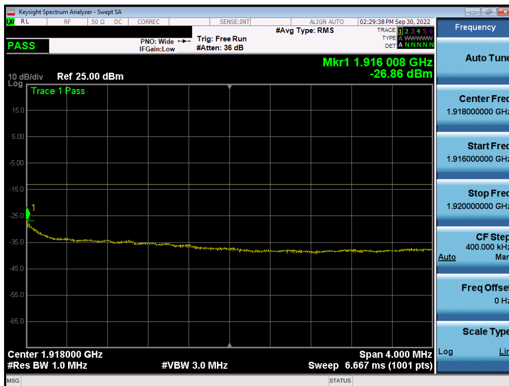
Plot 7-249. Extended Upper Band Edge Plot (NR Band n25 - 20MHz QPSK – Full RB - ANT F)
