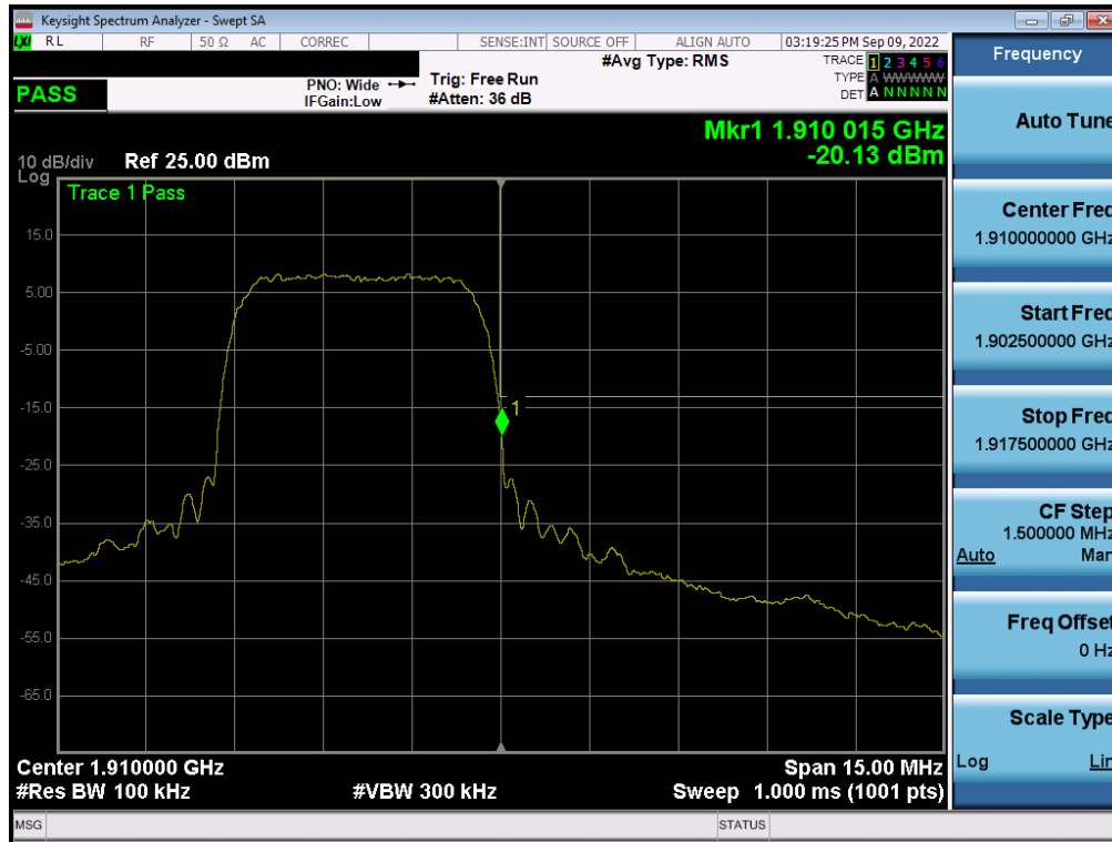
Plot 7-272. Upper Band Edge Plot (WCDMA PCS – Ch. 9538 - ANT A)
