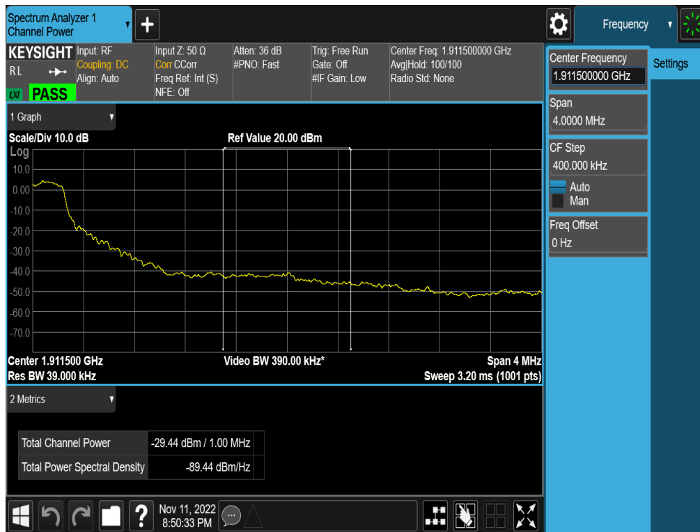
Plot 7-265. Extended Upper Band Edge Plot (NR Band n2 – 5MHz QPSK – Full RB - ANT F)
