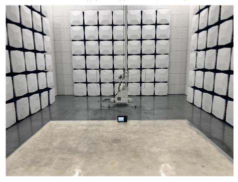
RADIATED EMISSION MEASUREMENT (Above 1G)
