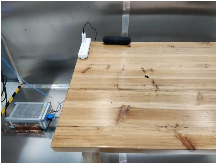
Photograph 1: Set-up for Conducted Emission on AC Mains
