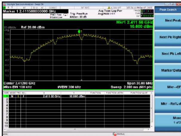
802.11b LOW CHANNEL, CARRIER LEVEL
