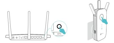
2. Wait until the Signal LED ((A)) changes to solid on, which indicates that the WPS connection is successful.
