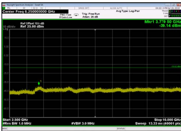
Conducted Emission: pi/4DQPSK,2402,2DH5 ,2500MHz~10000MHz
