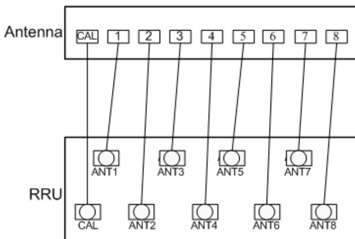
**Figure 8-14** Mapping relationship between the RF ports and the antenna ports2
