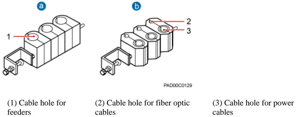
The following figure shows the cables secured on a cable tray.
