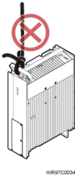
**Figure 6-5** Forbidding hoisting an RRU by the traction eye only
