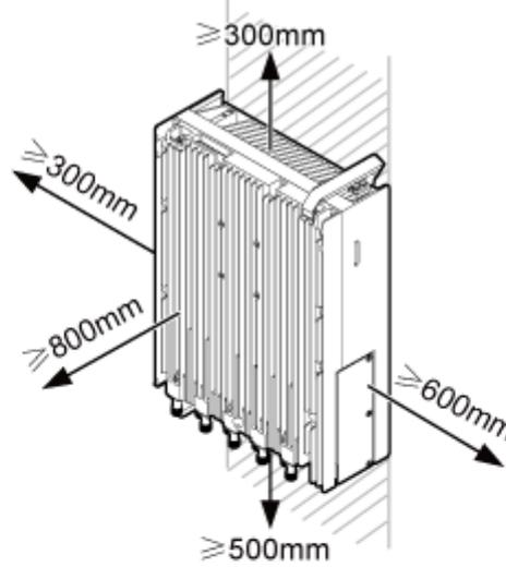
**Minimum clearance for installing an RRU**
