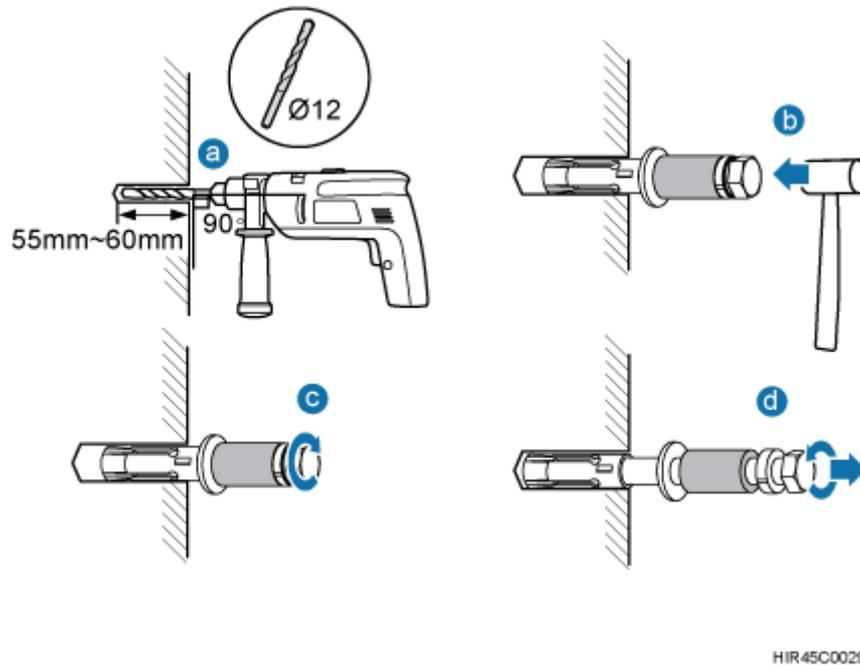
1. Use a hammer drill with a  $\Phi 12$  bit to drill holes vertically at the marked anchor points. Ensure that the depth of each hole ranges from 55 mm (2.17 in.) to 60 mm (2.36 in.). Use a vacuum cleaner to clear the dust out from inside and around the holes, and measure the distances between holes. If any of the holes is beyond the acceptable range, mark a new anchor point and drill a new hole.
