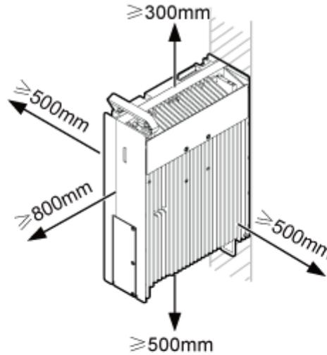
**Minimum clearance for installing an RRU**
