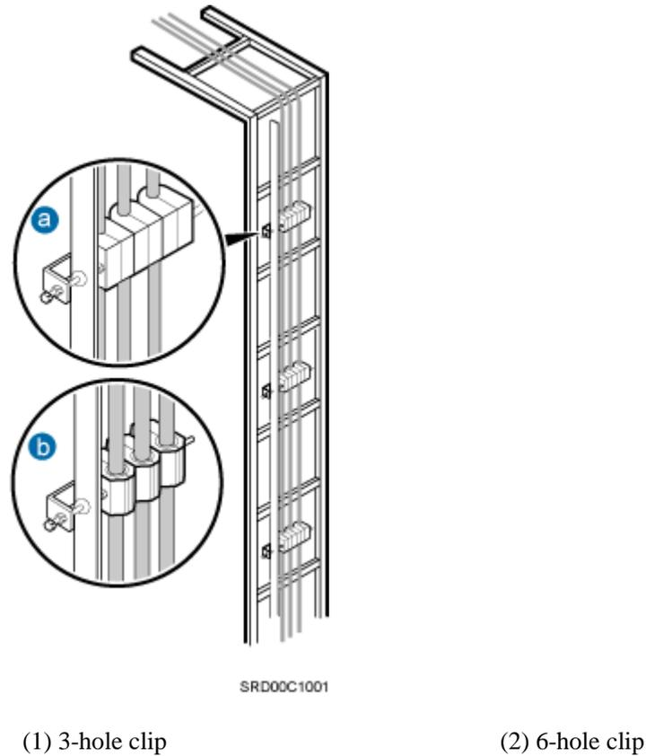
The following figure shows the cables secured on a tower.
