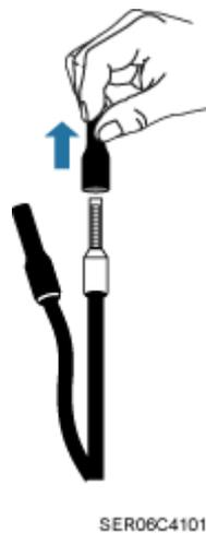
**Figure 8-24** Method for handling cord end terminals that are not in use
