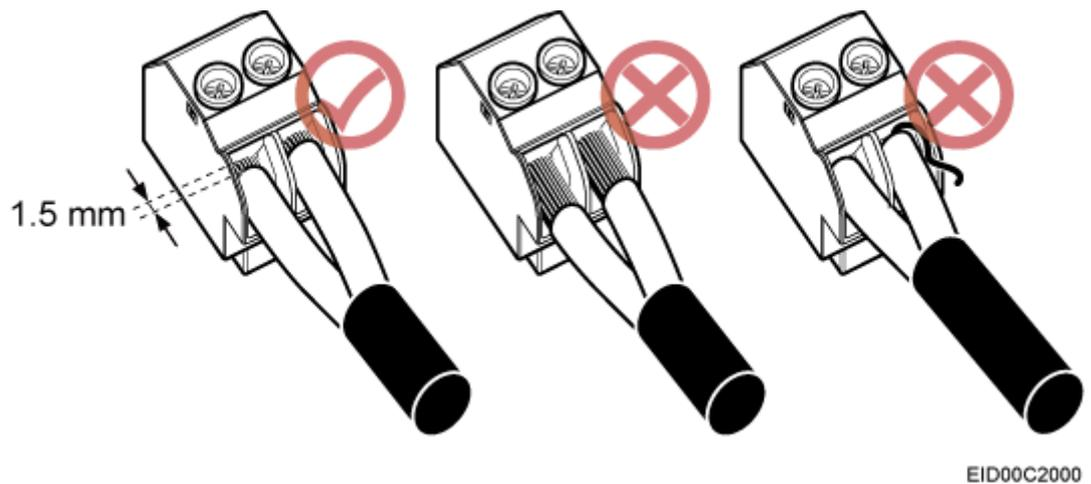
**Step 7** Pull the power cable with 30 N. Ensure that the core wires are securely connected to cord end terminals and there are no exposed conductor wires or copper wires, as shown in Figure 11-10.
