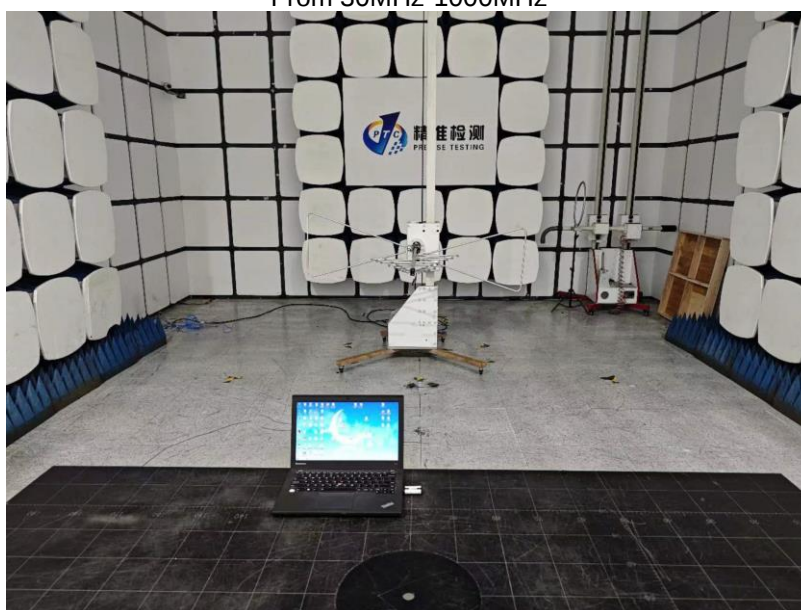
Radiated Spurious Emissions From 30MHz-1000MHz
