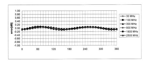
Axial Isotropy Error < ± 0.2 dB
