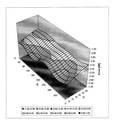
Spherical Isotropy Error < ± 0.4 dB
