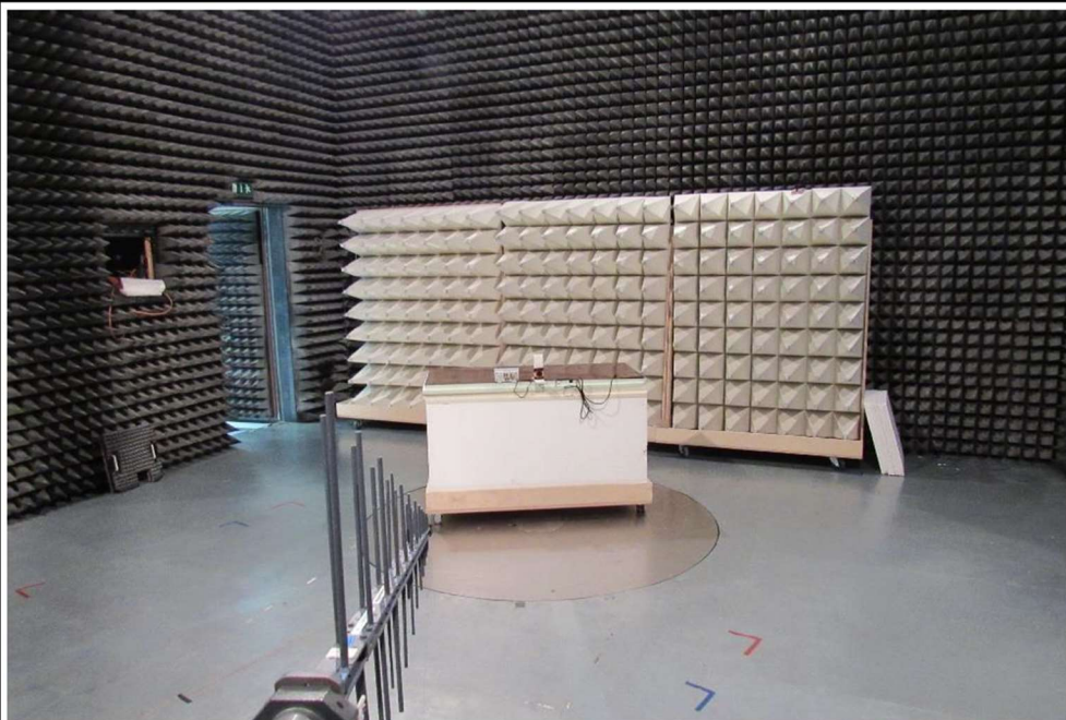
Test Setup Radiated Emissions 200 - 1000 MHz
