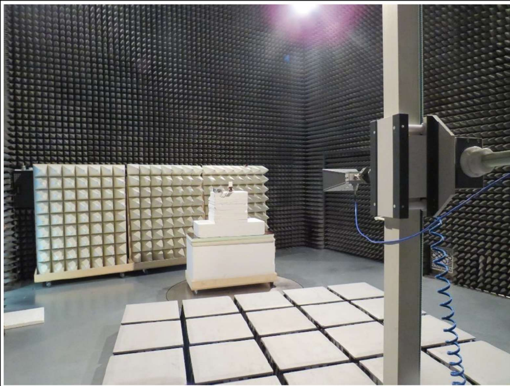
Test Setup Radiated Emissions 1 - 6.5 GHz
