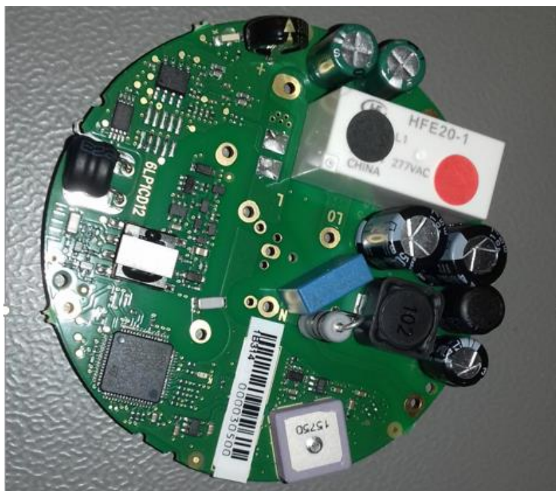
Figure 3 Main PCB top varistor removed
