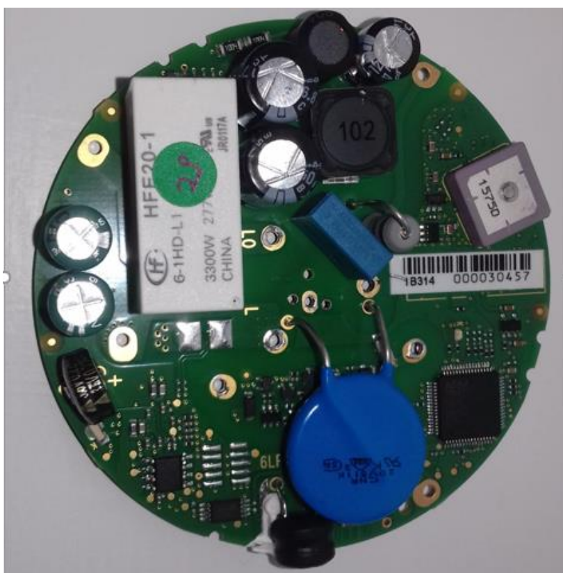
Figure 4 Main PCB top including varistor
