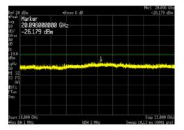
LTE20 Channel Bandwidth \_ QPSK \_ Middle Channel (1962.5MHz) at 40 watts/carrier:
