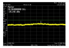
LTE20 Channel Bandwidth \_ 256QAM \_ Middle Channel (1962.5MHz) at 40 watts/carrier:
