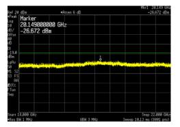
LTE15 Channel Bandwidth \_ 64QAM \_ Middle Channel (1962.5MHz) at 40 watts/carrier:
