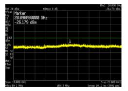
LTE5 Channel Bandwidth \_ QPSK \_ Middle Channels (1962.5MHz and 2145MHz) at 20W/Carrier:
