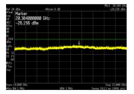
LTE15 Channel Bandwidth \_ 256QAM \_ Middle Channel (1962.5MHz) at 40 watts/carrier:
