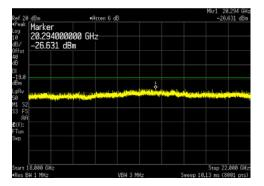
LTE20 Channel Bandwidth \_ 16QAM \_ Middle Channel (1962.5MHz) at 40 watts/carrier:
