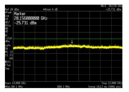
LTE5 Channel Bandwidth \_ 64QAM \_ Middle Channels (1962.5MHz and 2145MHz) at 20W/Carrier:
