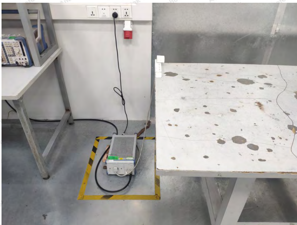
Photo of Power Line Conducted Emission Test
