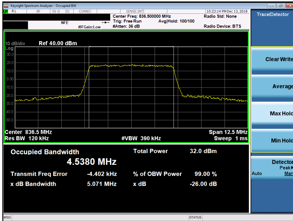
Plot 7-13. Occupied Bandwidth Plot (Band 5 - 5.0MHz QPSK - Full RB Configuration)
