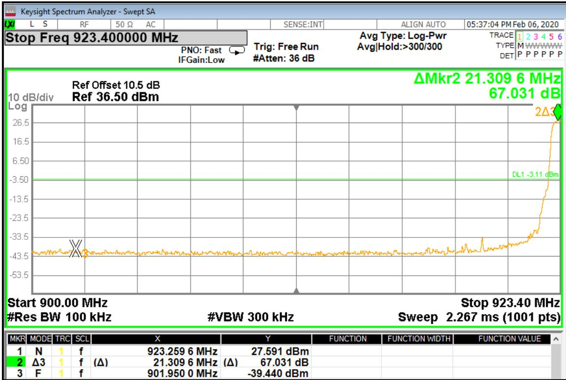
Screen Capture from the spectrum analyzer: Upper Band Edge (500 KHz DTS Mode)
