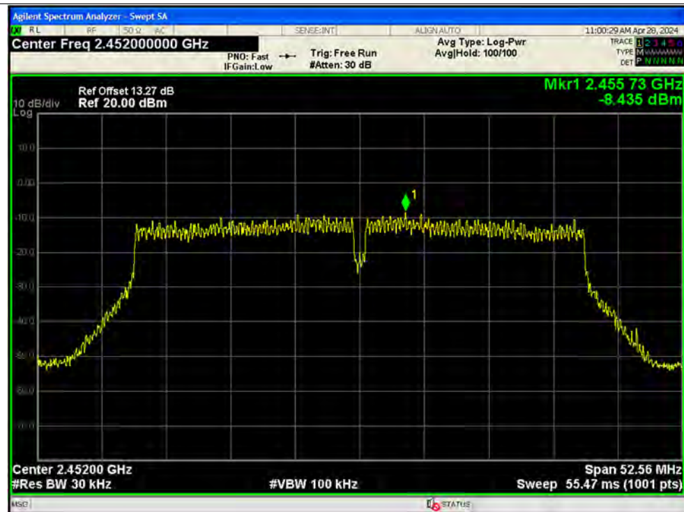
PSD NVNT ac40 2452MHz Ant1
