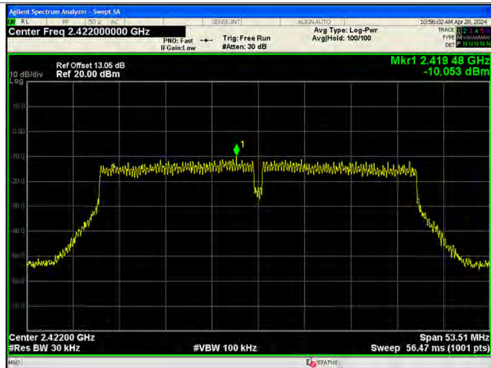
PSD NVNT ac40 2422MHz Ant1
