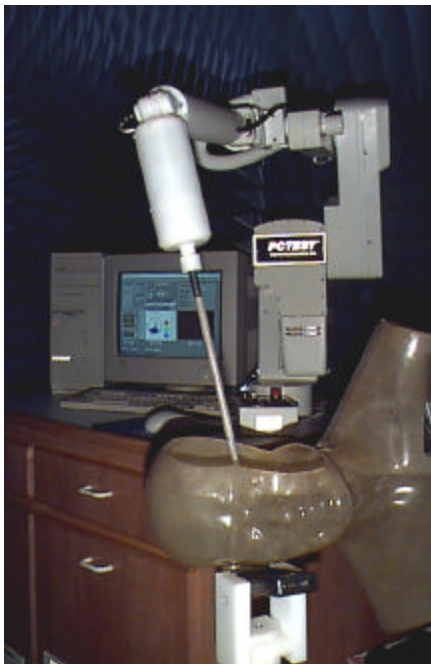
Figure 5. Photograph of the Probe and the Phantom
