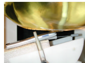
Fig. 17 Head SAR Test Setup
