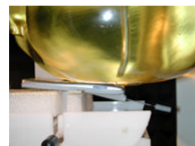
Fig. 16 Head SAR Test Setup
