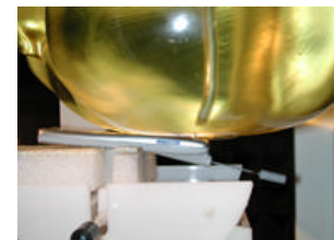
Fig. 21 Head SAR Test Setup
