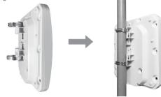
Anchor ear's diameter should be 33-57mm.
