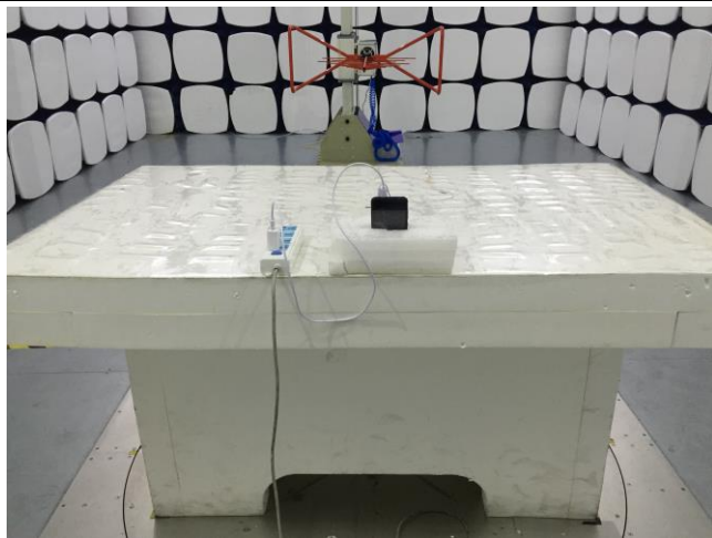
Conducted Emissions Test Setup Front View
