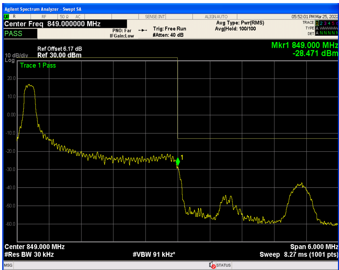
Band5 QPSK BW=3MHz Channel=20635 RB Size=1 Position=#Max
