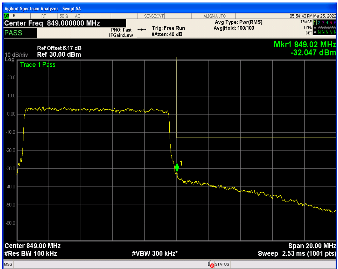
Band7 QPSK BW=5MHz Channel=20775 RB Size=1 Position=#0
