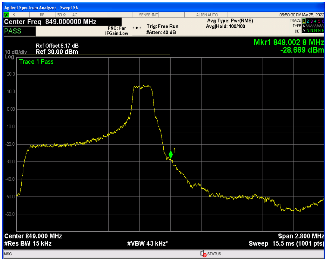
Band5 QAM16 BW=1.4MHz Channel=20643 RB Size=1 Position=#0
