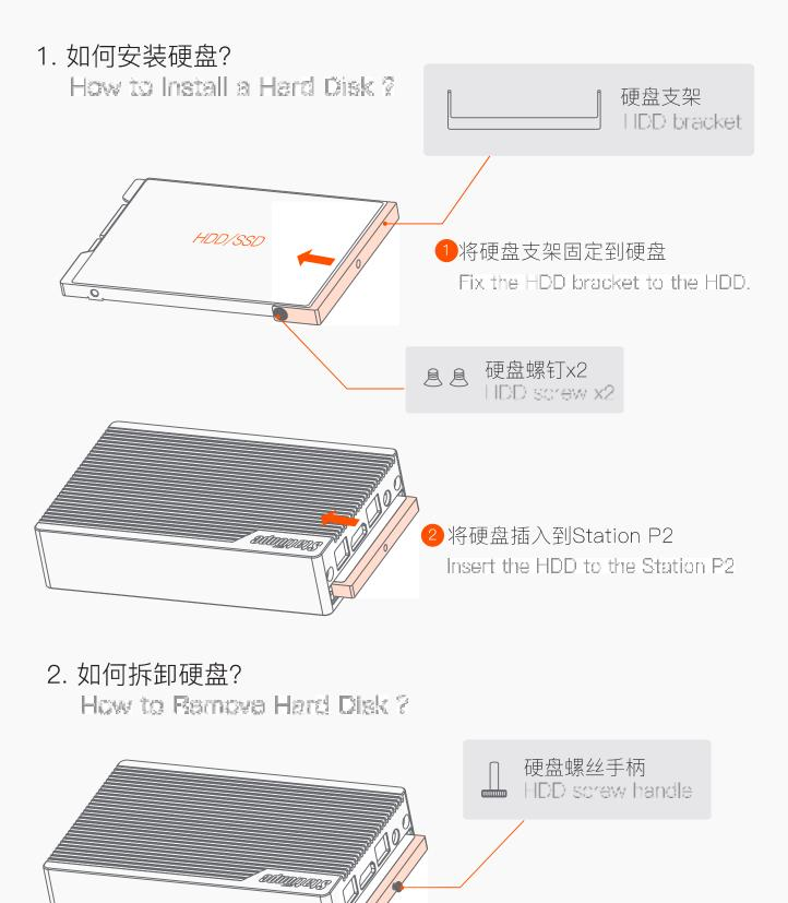
1 把硬盘螺丝手柄拧到硬盘支架 的螺丝孔上,即可抽出硬盘 Install HDD screw handle to HDD bracket; pull out Hard Disk.
