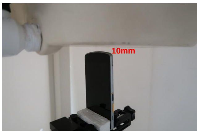
Bottom Side, Test Separation 10 mm
