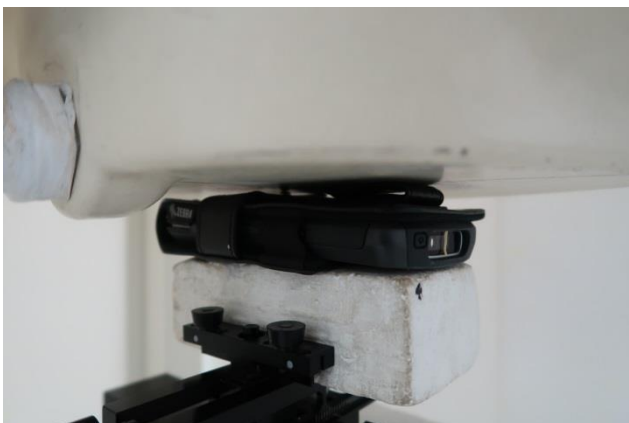
Front with Soft Holster + Rigid Holster, Test Separation 0 mm
