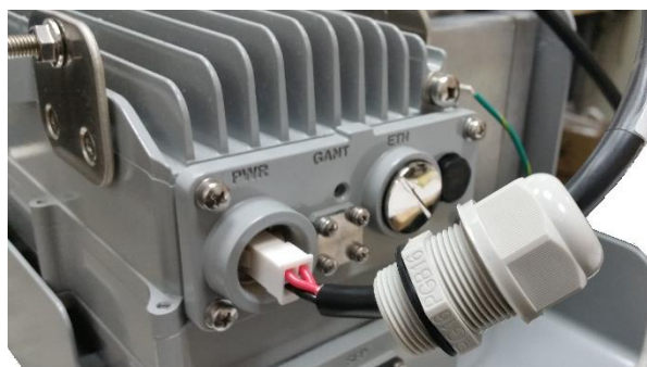
Figure 30: Attach Power cable
