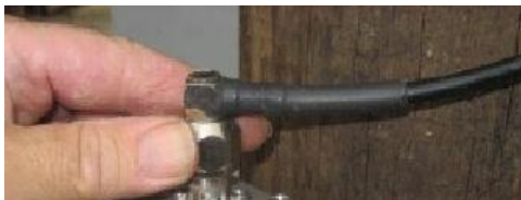
Figure 32: Connecting RF cable
