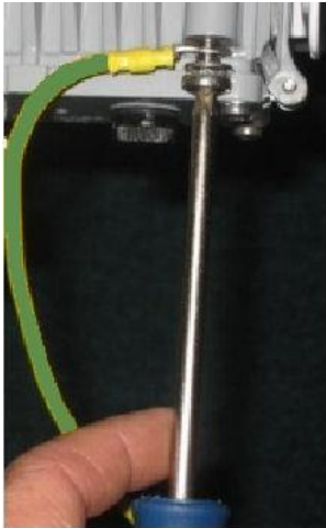
Figure 21: Attaching ground cable to AirHarmony-1000D
