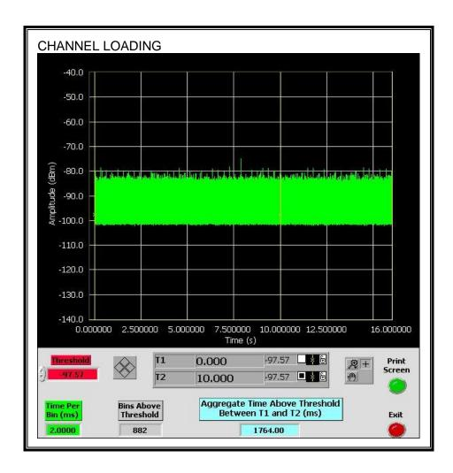
The level of traffic loading on the channel by the EUT is 17.64%
