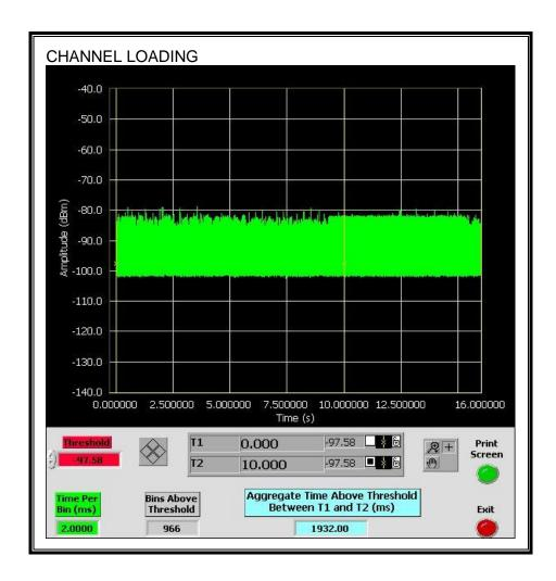
The level of traffic loading on the channel by the EUT is 19.32%
