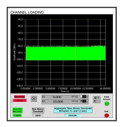
The level of traffic loading on the channel by the EUT is 20.4%
