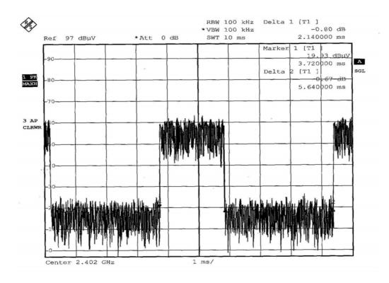
$$20\log(\text{Duty cycle}) = 20\log\frac{2.14 \text{ ms}}{5.64 \text{ ms}} = -8.4 \text{dB}$$
