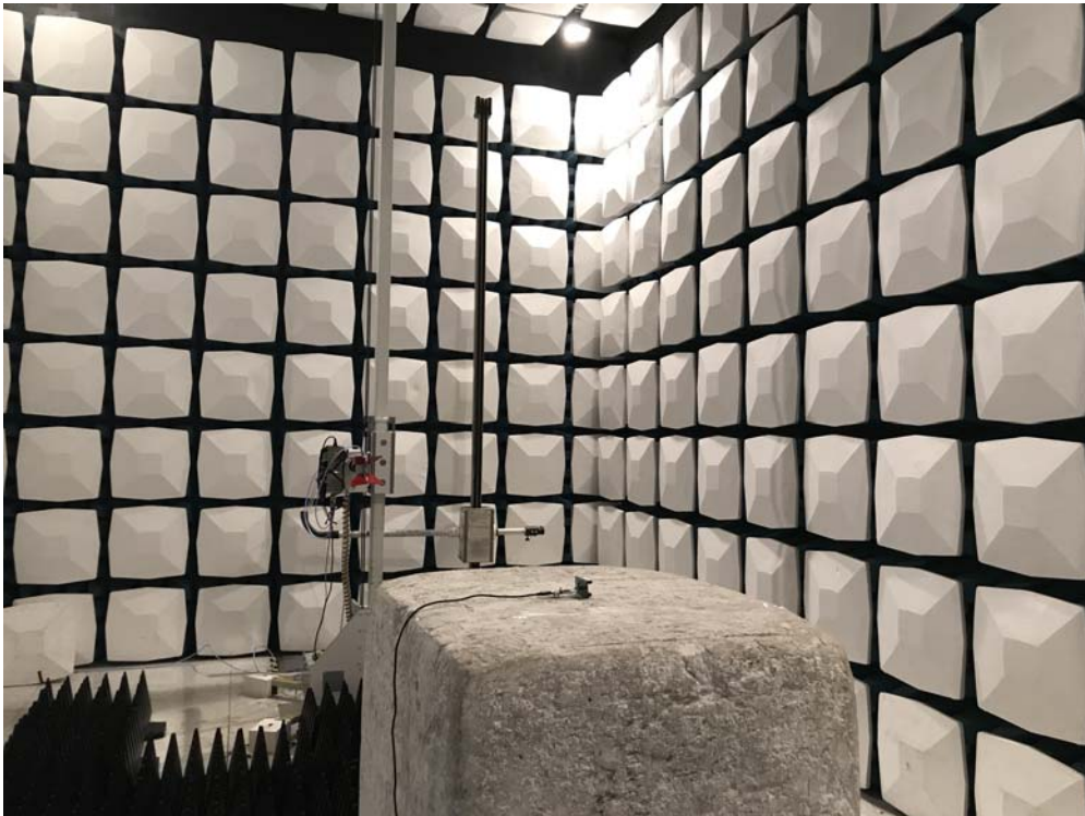
Description: Radiated Emission Test Setup for 1~18GHz
