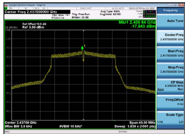
Power spectral density-802.11n(HT20) ,2437MHz,Ant0
