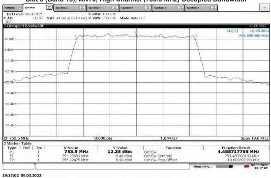
TM1.1-QPSK\_5 MHz Bandwidth (4G LTE) With RP5100 Host Slot 0 (Band 13), ANT1, High Channel (753.5 MHz) Occupied Bandwidth
