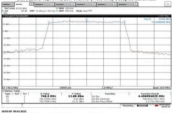
TM3.1-64QAM\_5 MHz Bandwidth (4G LTE) With RP5100 Host Slot 0 (Band 13), ANT1, Low Channel (748.5 MHz) Occupied Bandwidth
