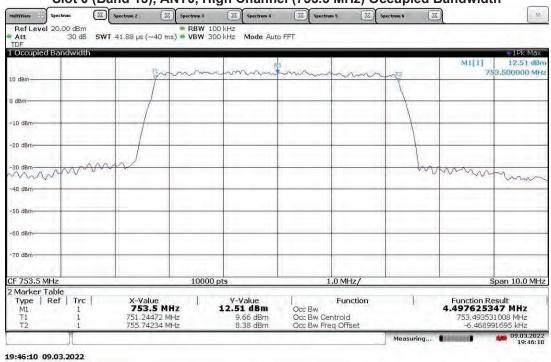
TM3.1a-256QAM\_5 MHz Bandwidth (4G LTE) With RP5100 Host Slot 0 (Band 13), ANT1, High Channel (753.5 MHz) Occupied Bandwidth
