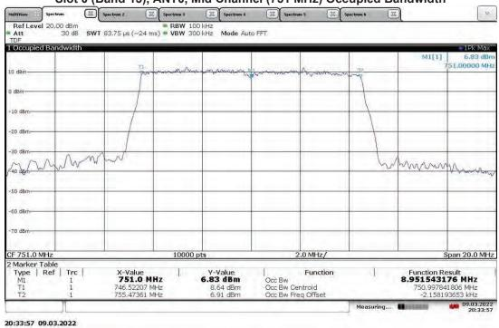
TM3.1a-256QAM\_10 MHz Bandwidth (4G LTE) With RP5100 Host Slot 0 (Band 13), ANT1, Mid Channel (751 MHz) Occupied Bandwidth
