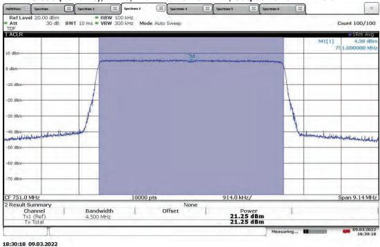
TM1.1-QPSK\_5 MHz Bandwidth (4G LTE) With RP5100 Host Slot 0 (Band 13), ANT1, Mid Channel 751 MHz, Output Power = 20.89 dBm
