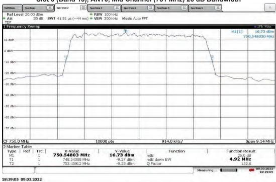
TM3.2-16QAM\_5 MHz Bandwidth (4G LTE) With RP5100 Host Slot 0 (Band 13), ANT1, Mid Channel (751 MHz) 26 dB Bandwidth
