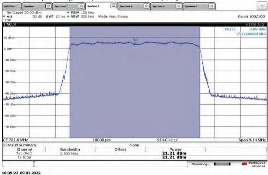
TM3.2-16QAM\_5 MHz Bandwidth (4G LTE) With RP5100 Host Slot 0 (Band 13), ANT1, Mid Channel 751 MHz, Output Power = 20.86 dBm
