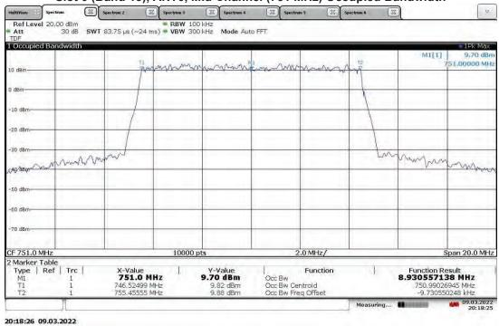
TM3.2-16QAM\_10 MHz Bandwidth (4G LTE) With RP5100 Host Slot 0 (Band 13), ANT1, Mid Channel (751 MHz) Occupied Bandwidth
