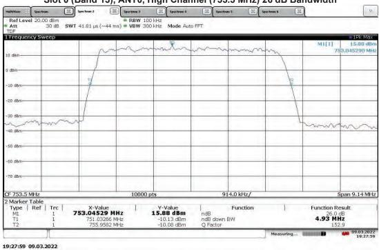
TM3.2-16QAM\_5 MHz Bandwidth (4G LTE) With RP5100 Host Slot 0 (Band 13), ANT1, High Channel (753.5 MHz) 26 dB Bandwidth
