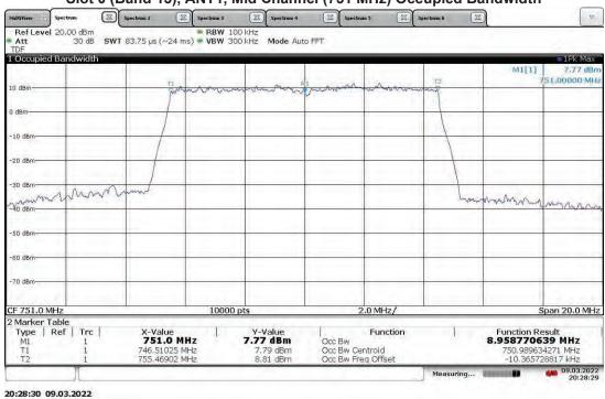
TM3.1a-256QAM\_10 MHz Bandwidth (4G LTE) With RP5100 Host Slot 0 (Band 13), ANT0, Mid Channel (751 MHz) Occupied Bandwidth
