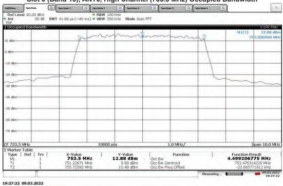
TM3.2-16QAM\_5 MHz Bandwidth (4G LTE) With RP5100 Host Slot 0 (Band 13), ANT1, High Channel (753.5 MHz) Occupied Bandwidth
