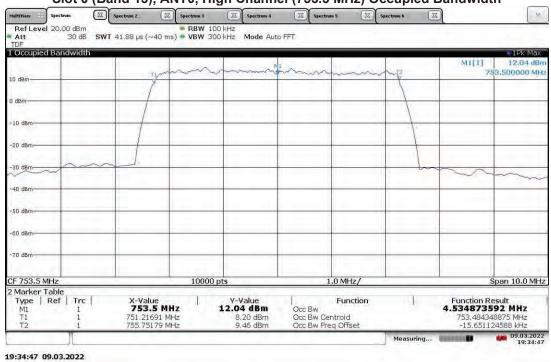
TM3.1-64QAM\_5 MHz Bandwidth (4G LTE) With RP5100 Host Slot 0 (Band 13), ANT1, High Channel (753.5 MHz) Occupied Bandwidth
