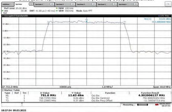
TM1.1-QPSK\_5 MHz Bandwidth (4G LTE) With RP5100 Host Slot 0 (Band 13), ANT1, Mid Channel (751 MHz) Occupied Bandwidth
