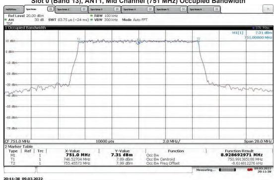
TM3.2-16QAM\_10 MHz Bandwidth (4G LTE) With RP5100 Host Slot 0 (Band 13), ANT0, Mid Channel (751 MHz) Occupied Bandwidth
