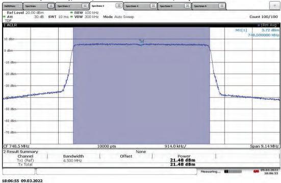
TM3.1-64QAM\_5 MHz Bandwidth (4G LTE) With RP5100 Host Slot 0 (Band 13), ANT1, Low Channel 748.5 MHz, Output Power = 20.76dBm
