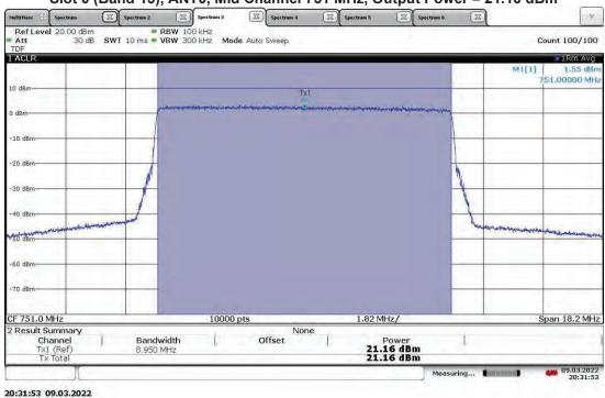
TM3.1-64QAM\_10 MHz Bandwidth (4G LTE) With RP5100 Host Slot 0 (Band 13), ANT1, Mid Channel 751 MHz, Output Power = 20.83 dBm
