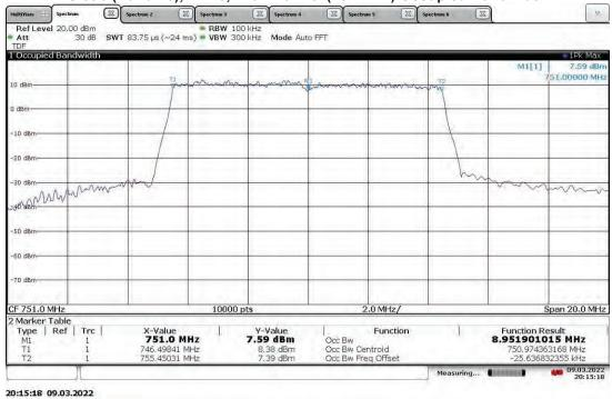
TM1.1-QPSK\_10 MHz Bandwidth (4G LTE) With RP5100 Host Slot 0 (Band 13), ANT1, Mid Channel (751 MHz) Occupied Bandwidth
