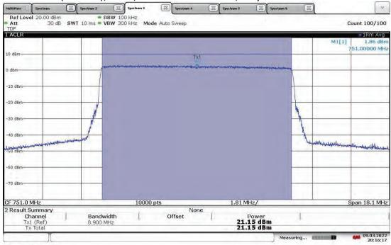
TM1.1-QPSK\_10 MHz Bandwidth (4G LTE) With RP5100 Host
