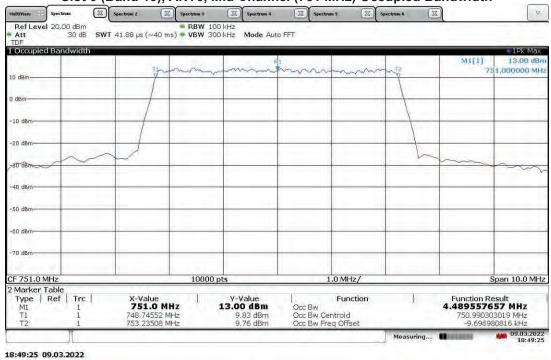
TM3.1a-256QAM\_5 MHz Bandwidth (4G LTE) With RP5100 Host Slot 0 (Band 13), ANT1, Mid Channel (751 MHz) Occupied Bandwidth
