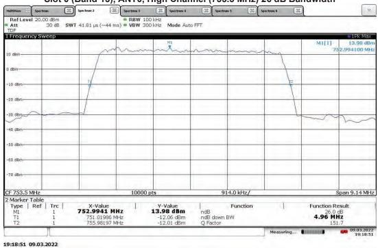
TM1.1-QPSK\_5 MHz Bandwidth (4G LTE) With RP5100 Host Slot 0 (Band 13), ANT1, High Channel (753.5 MHz) 26 dB Bandwidth
