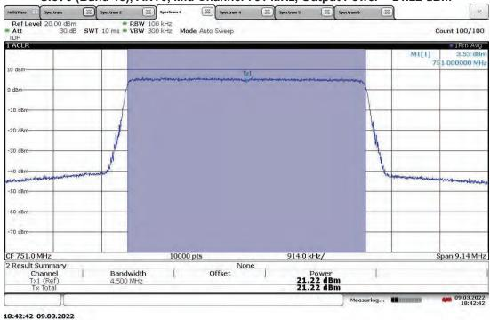
TM3.1-64QAM\_5 MHz Bandwidth (4G LTE) With RP5100 Host Slot 0 (Band 13), ANT1, Mid Channel 751 MHz, Output Power = 20.88 dBm
