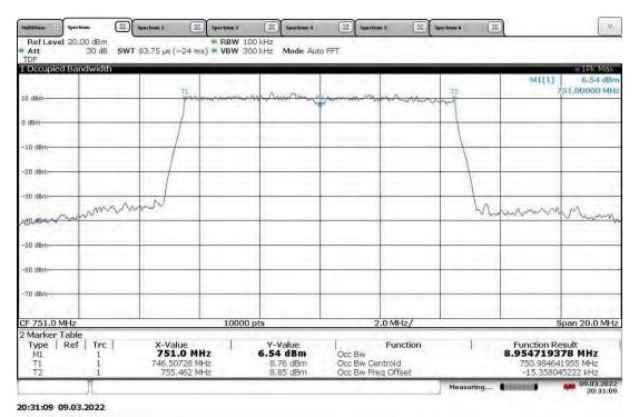
TM3.1-64QAM\_10 MHz Bandwidth (4G LTE) With RP5100 Host Slot 0 (Band 13), ANT1, Mid Channel (751 MHz) Occupied Bandwidth
