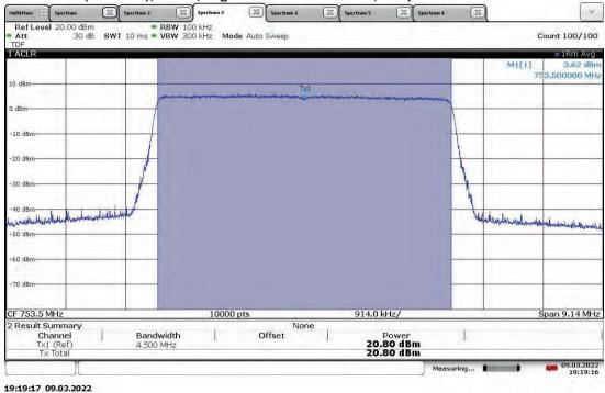
TM1.1-QPSK\_5 MHz Bandwidth (4G LTE) With RP5100 Host Slot 0 (Band 13), ANT1, High Channel 753.5 MHz, Output Power = 20.87 dBm
