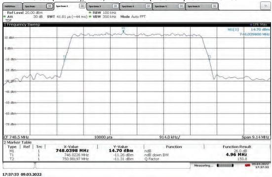
TM1.1-QPSK\_5 MHz Bandwidth (4G LTE) With RP5100 Host Slot 0 (Band 13), ANT1, Low Channel (748.5 MHz) 26 dB Bandwidth
