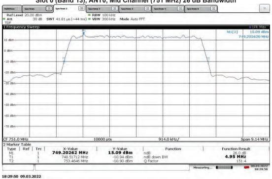
TM1.1-QPSK\_5 MHz Bandwidth (4G LTE) With RP5100 Host Slot 0 (Band 13), ANT1, Mid Channel (751 MHz) 26 dB Bandwidth
