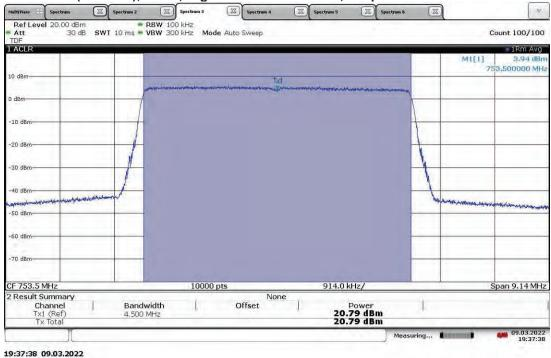
TM3.1-64QAM\_5 MHz Bandwidth (4G LTE) With RP5100 Host Slot 0 (Band 13), ANT1, High Channel 753.5 MHz, Output Power = 20.85 dBm
