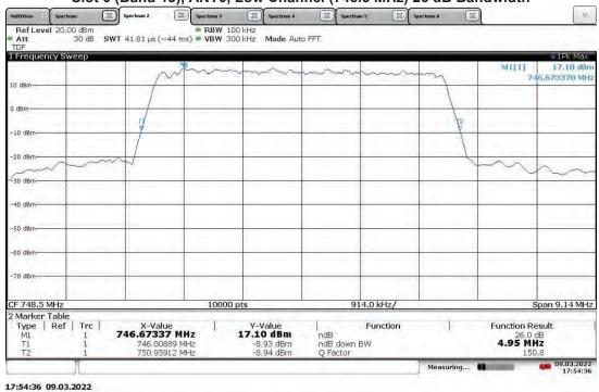
TM3.2-16QAM\_5 MHz Bandwidth (4G LTE) With RP5100 Host
