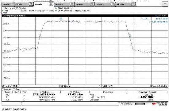
TM3.1-64QAM\_5 MHz Bandwidth (4G LTE) With RP5100 Host Slot 0 (Band 13), ANT1, Low Channel (748.5 MHz) 26 dB Bandwidth
