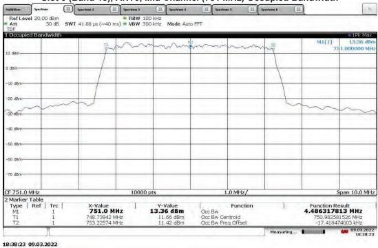
TM3.2-16QAM\_5 MHz Bandwidth (4G LTE) With RP5100 Host Slot 0 (Band 13), ANT1, Mid Channel (751 MHz) Occupied Bandwidth
