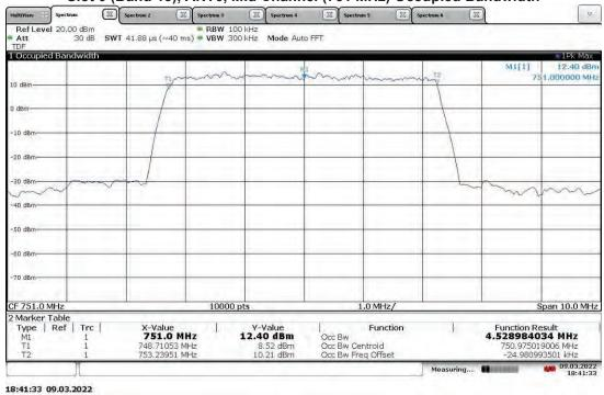
TM3.1-64QAM\_5 MHz Bandwidth (4G LTE) With RP5100 Host Slot 0 (Band 13), ANT1, Mid Channel (751 MHz) Occupied Bandwidth
