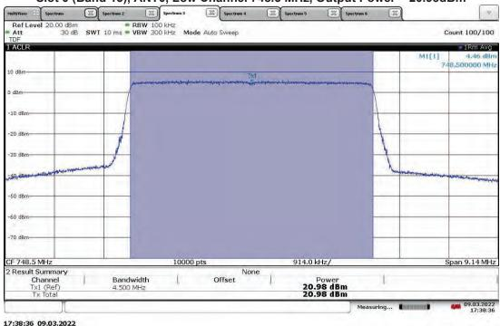
TM1.1-QPSK\_5 MHz Bandwidth (4G LTE) With RP5100 Host Slot 0 (Band 13), ANT1, Low Channel 748.5 MHz, Output Power = 20.29 dBm
