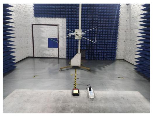
RADIATED EMISSION TEST SETUP ABOVE 1GHZ
