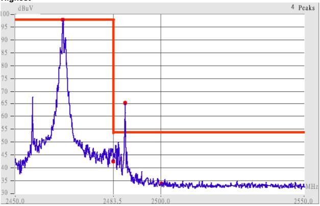
This is the hard copy of our bandedge measurement generated by our bandedge testing program. The plot shown above is the bandedge of highest channel.
