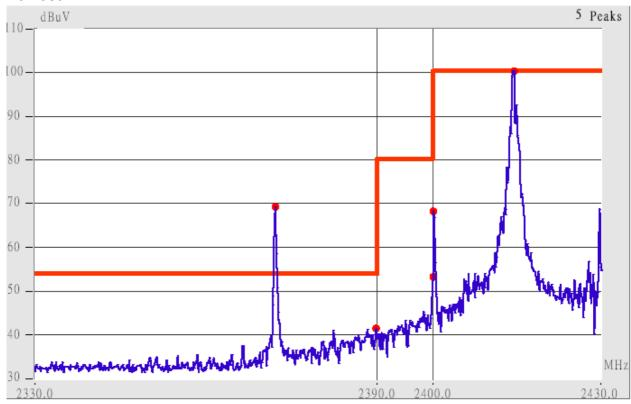
This is the hard copy of our bandedge measurement generated by our bandedge testing program. The plot shown above is the bandedge of lowest channel.
