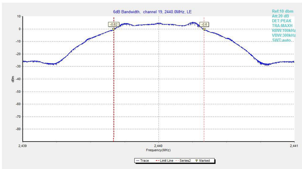
Fig.21. 6dB Bandwidth: GFSK, 2440 MHz
