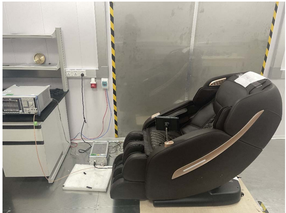
Conducted Emission Test Setup
