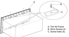
5. Release the 4 locating pins from locating holes, take out the trim kit frame, and set aside.
