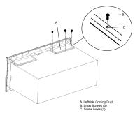
4. Loosen the 4 screws which fast the trim kit frame to the microwave oven, and set the 4 screws aside.
