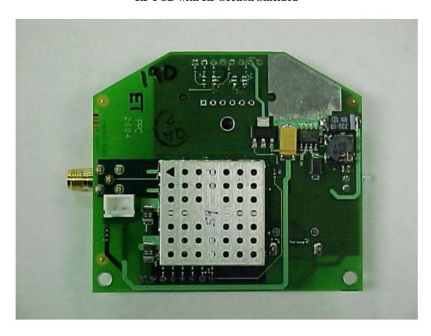
Vehicle Safety and Security Reporting System Vehicle Unit 902 – 928 MHz Radio
