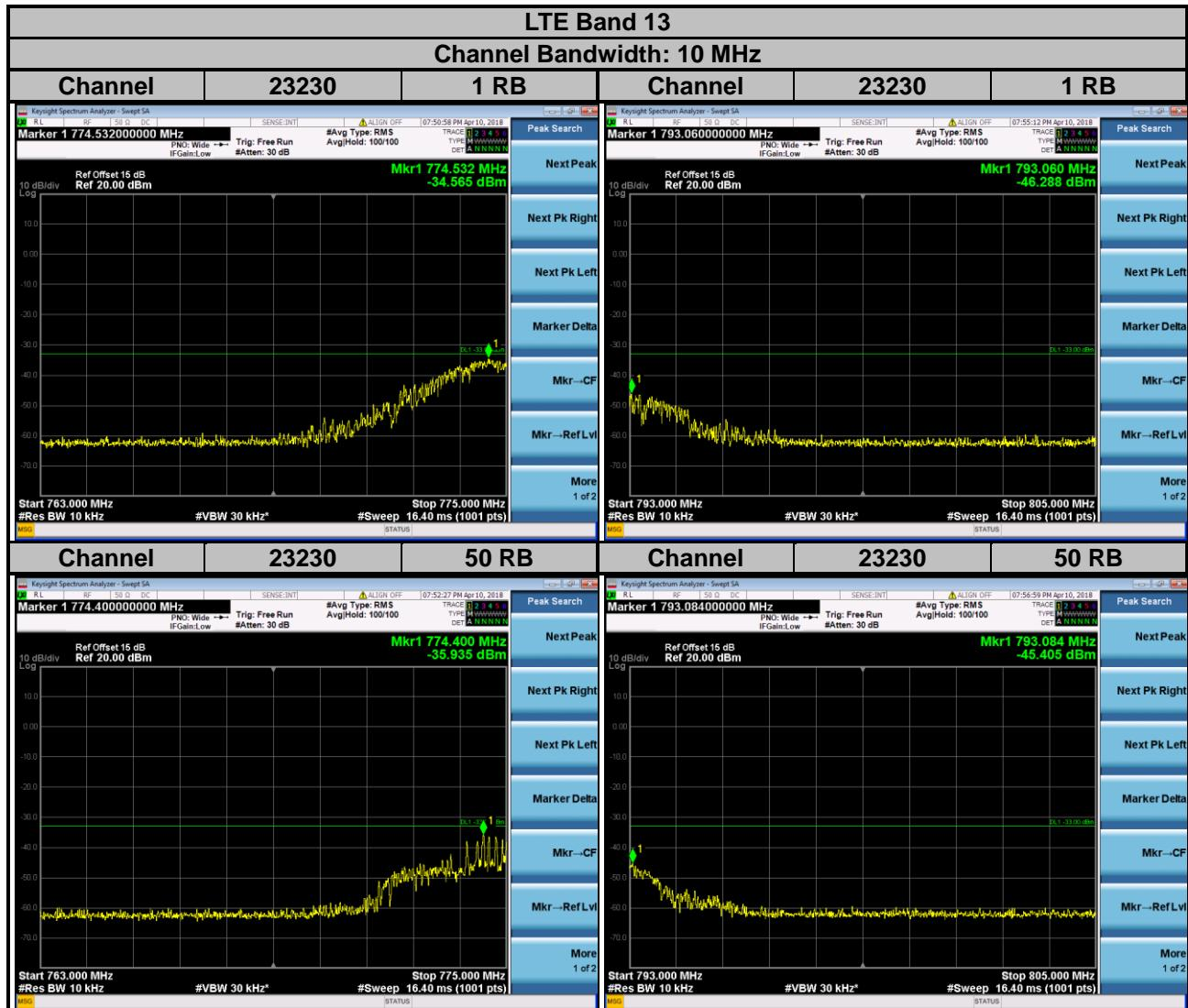
For the 763 - 775 MHz and 793 - 805 MHz band, the FCC limit is  $65 + 10\log(P[\text{watt}])$  in a 6.25 kHz bandwidth. Since it was not possible to set the resolution bandwidth to 6.25 kHz with the available equipment, a bandwidth of 10 kHz was used instead to show compliance. By using a 10 kHz bandwidth on the spectrum analyzer.
