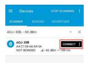
3. Turn on the Bluetooth receiving service, as shown in Figure 3; measure once normally to check whether the Bluetooth has received data, as shown in Figure 4;
