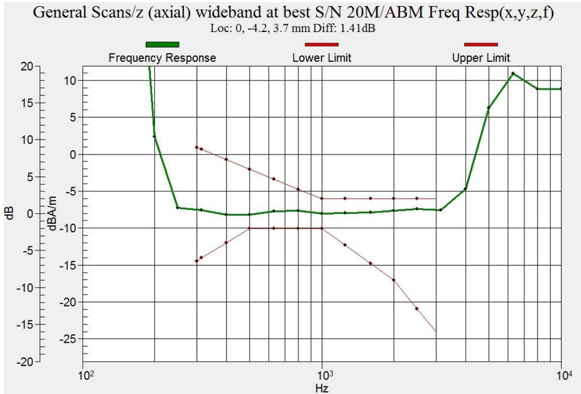
**Figure C.14 Frequency Response of LTE B71**
