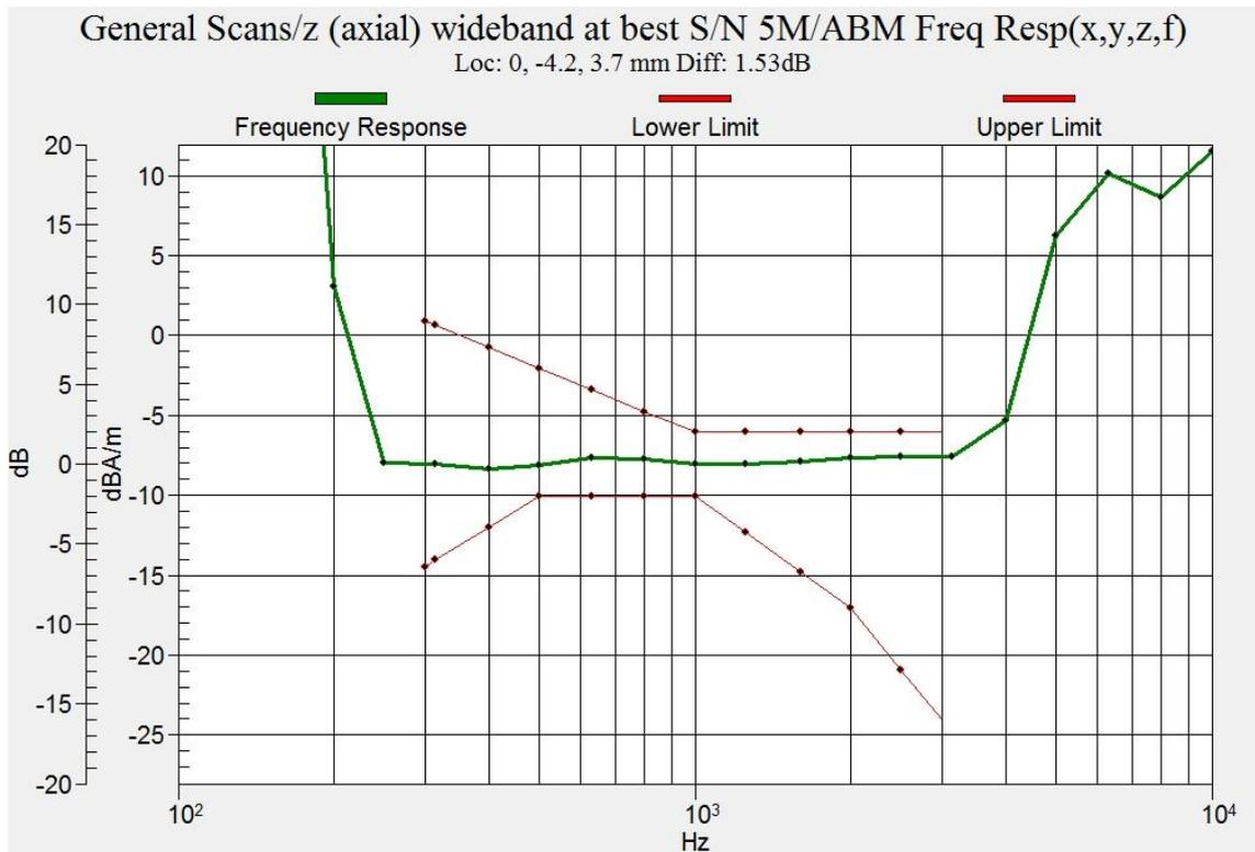
**Figure C.9 Frequency Response of LTE B12**
