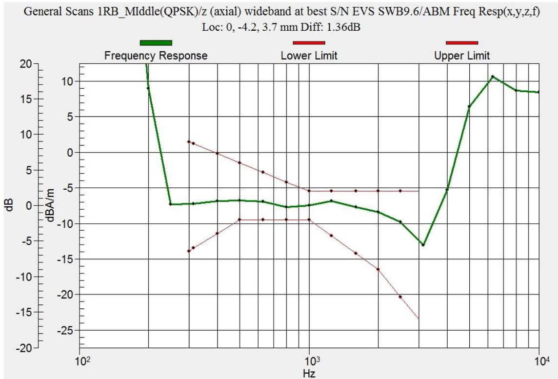
**Figure C.6 Frequency Response of LTE B2**
