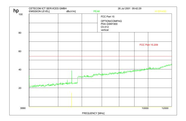
Carrier at 5550 MHz is 42.5 dBµV/m Peak and 18.9 dBµV/m Average at 3m distance.
