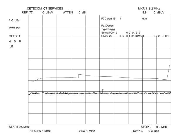
Carrier is notched with a Band Reject Filter
