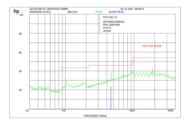
Carrier is notched with a Band Reject Filter.
