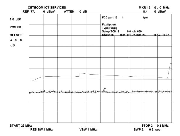
Carrier is notched with a Band Reject Filter.
